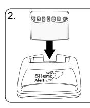
Install the trickle charger (Part no. CCT3A-2214-IN), insert the Pager into the charging slot and charge for 24 hours. The battery key on the Pager will light green briefly upon docking and the sounder will beep 3 times confirming the Pager is docked correctly.
