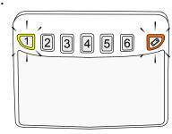
If the low battery sequence alternates with another zone key the monitor configured to send that zone has a low battery. Replace the Monitor battery and transmit to test.
